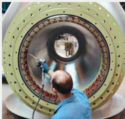
Preparation of an insulated and impregnated generator for a wind turbine
